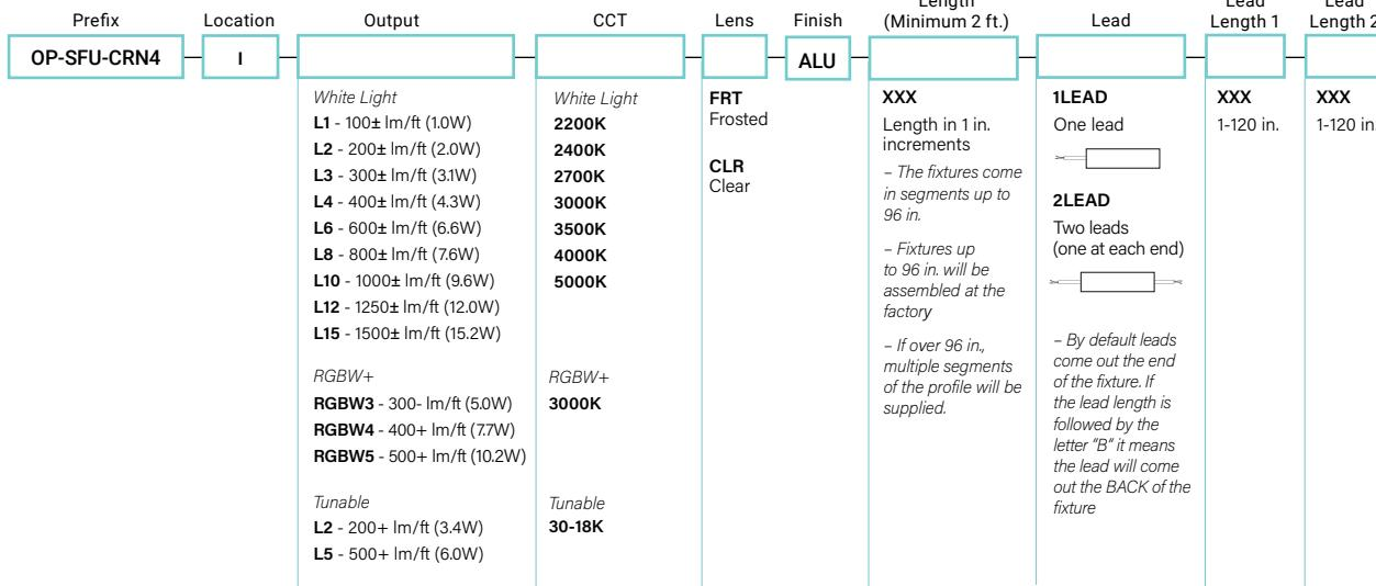
Fixtures are supplied with Optique's remote Universal power supply supporting 0-10, 1-10V, MLV, ELV dimming and voltage input from 100V-277V.
