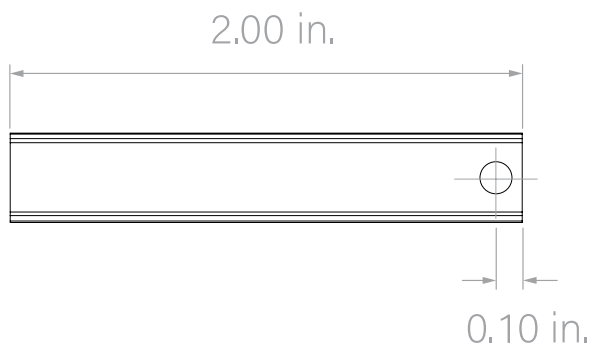
Factory Pre-Wired End Piece Back View Dimensions
