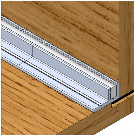
Millwork - Surface Mount - 90° Mounting Angle is designed with woodwork and millwork in mind. This innovative luminaire seamlessly integrates into the underside of shelves, counters, and desks, delivering refined, direct downward lighting. Engineered for effortless installation with a V-groove drill guide for power access and retention ridges that securely hold the light engine in place.
