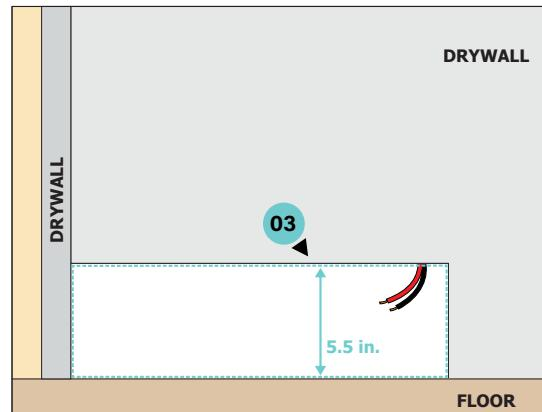
NOTE: It may be necessary to remove material from the backing plate or channel to run the power to the fixture.
