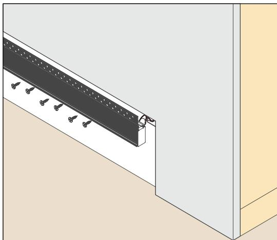
NOTE: Cover the fixture inside with painter's tape before plastering to prevent plaster and dust entering inside the fixture.
